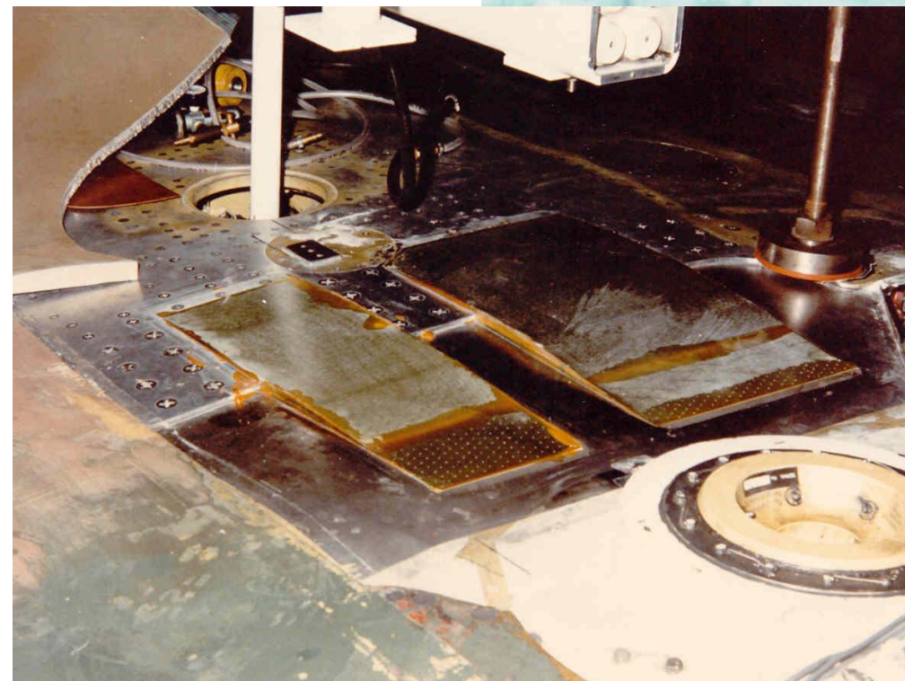
Boron/Epoxy Strengthening Doublers [14,16]
