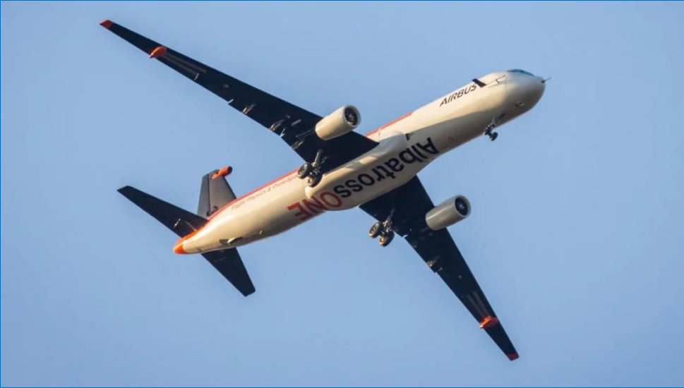
2019 Airbus Albatros one - Scale model flight test. Wing Aspect Ratio 18
