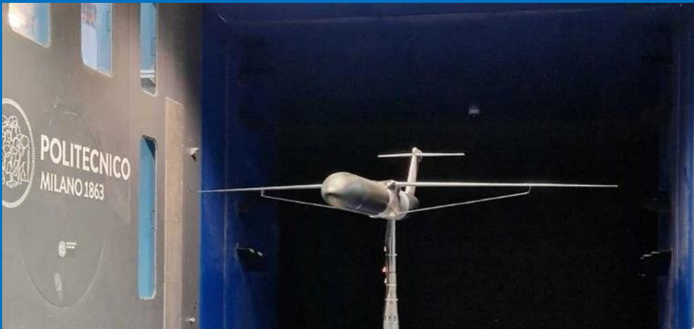
2022 EU CS2 U-HARWARD - Ultra High Aspect Ratio Wing Advanced Research and Designs Wing Aspect Ratio 15-20
