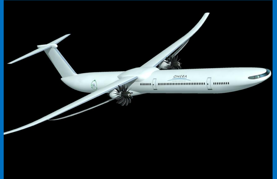
2023 ONERA Project Gullhyver: RISE Open Rotor, TTBW with Aspect Ratio of 20, 200 seats, 7500 km (Hydrogen but also usable for SAF)
