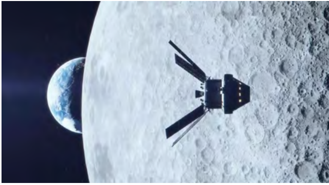
Figure 3 Solar arrays are folded backwards by 35 degrees. © NASA
